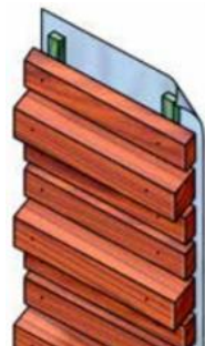
Figure 3 - Variable dimensions of horizontal open trapezium-shaped façade cladding for good drainage. (Source: Centrum Hout, 2024)
