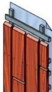
Figure 5 - Vertical open façade cladding (Source: Centrum Hout, 2024)
