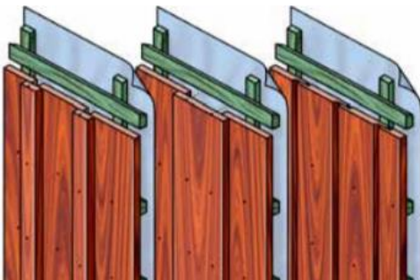
Figure 4 - Vertical cladding LTR: board & batten, board & batten and rebate with shiplap overlap (channel siding). (Source: Centrum Hout, 2024)
