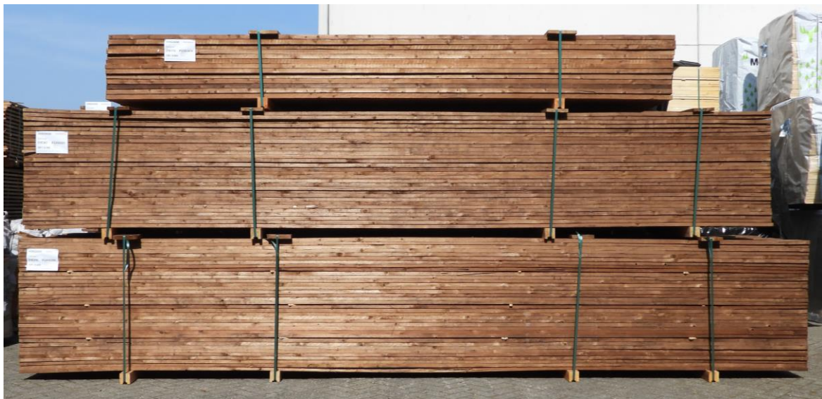
Figure 1 - Store the stacked untreated wood correctly
